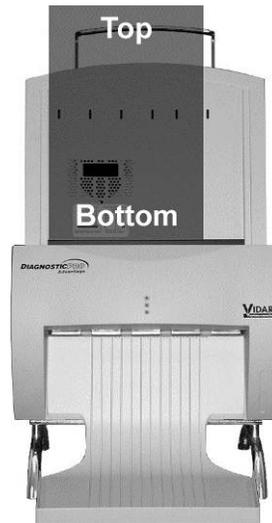
When the digitizer senses the film, it automatically stages the film in preparation for digitizing. The film will first move down, then up. This is normal operation.
