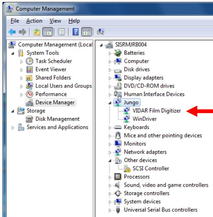
When using Window 7 & 8 32 Bit OS the Digitizer will be listed under **Imaging Devices**
