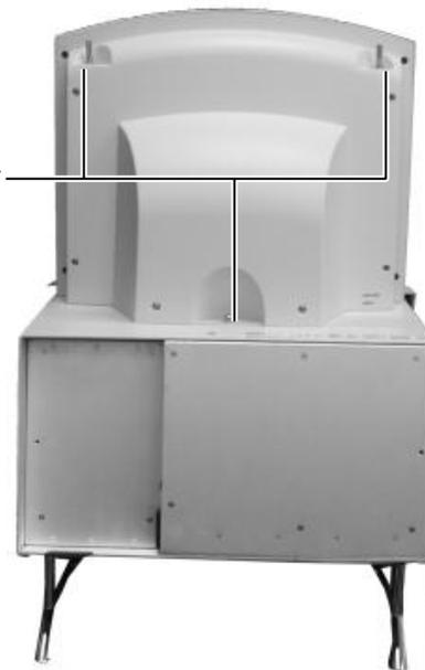
4. Install the exit tray by hooking it over the notched plastic edge just below the rollers. When the exit tray is properly positioned, it will be parallel to the roller shaft.
