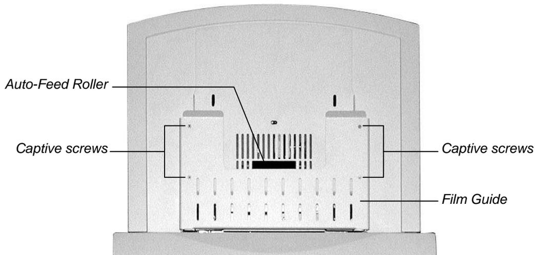
3. Remove residue from the Auto-Feed Roller: Loop a piece of light adhesive tape (such as Scotch® Magic™ Tape) around your fingers with the adhesive side out, then gently pat the roller. Pat and turn the roller until its entire surface is clean.
