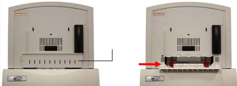
3. Set sliding film guide to proper width:
