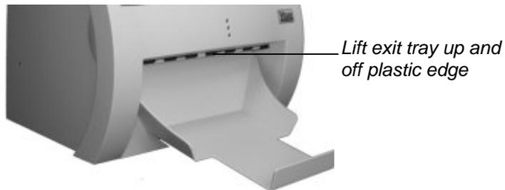
*Removing CAD PRO<sup>®</sup> Advantage exit tray*
