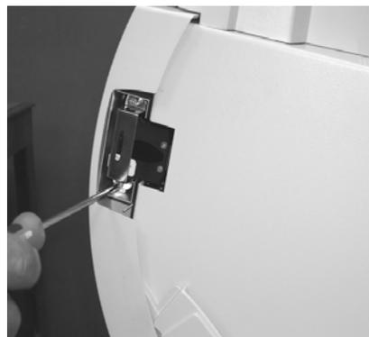
**Note:** The door has a “door open” sensor. When the door is open, all processes—including calibration and scanning—will stop.
